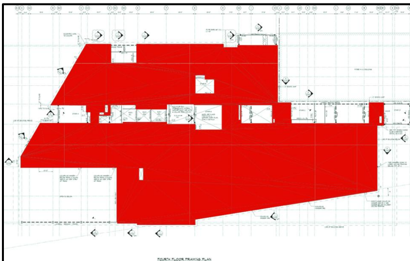
Figure 4 to the Left: Quantity Takeoff of the Type 6.25 slab on deck for the 4 th floor of the MMAA.
